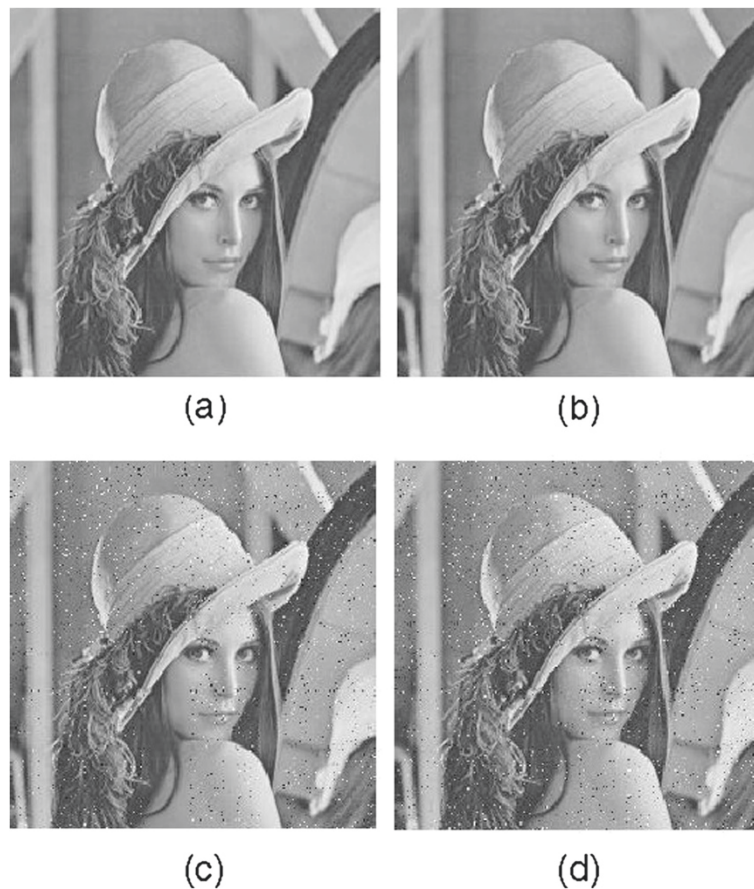
Figure 9 Image source 2 with \bar{p} = 0.62 at E_b/N_0 = 3.2 dB (a) transmitted image (b) proposed 2D system (0% pixel errors, PSNR \infty dB) (c) proposed 1D system (9.39% pixel errors, PSNR 39.97 dB) (d) conventional TBC system (11.52% pixel errors, PSNR 38.98 dB).
