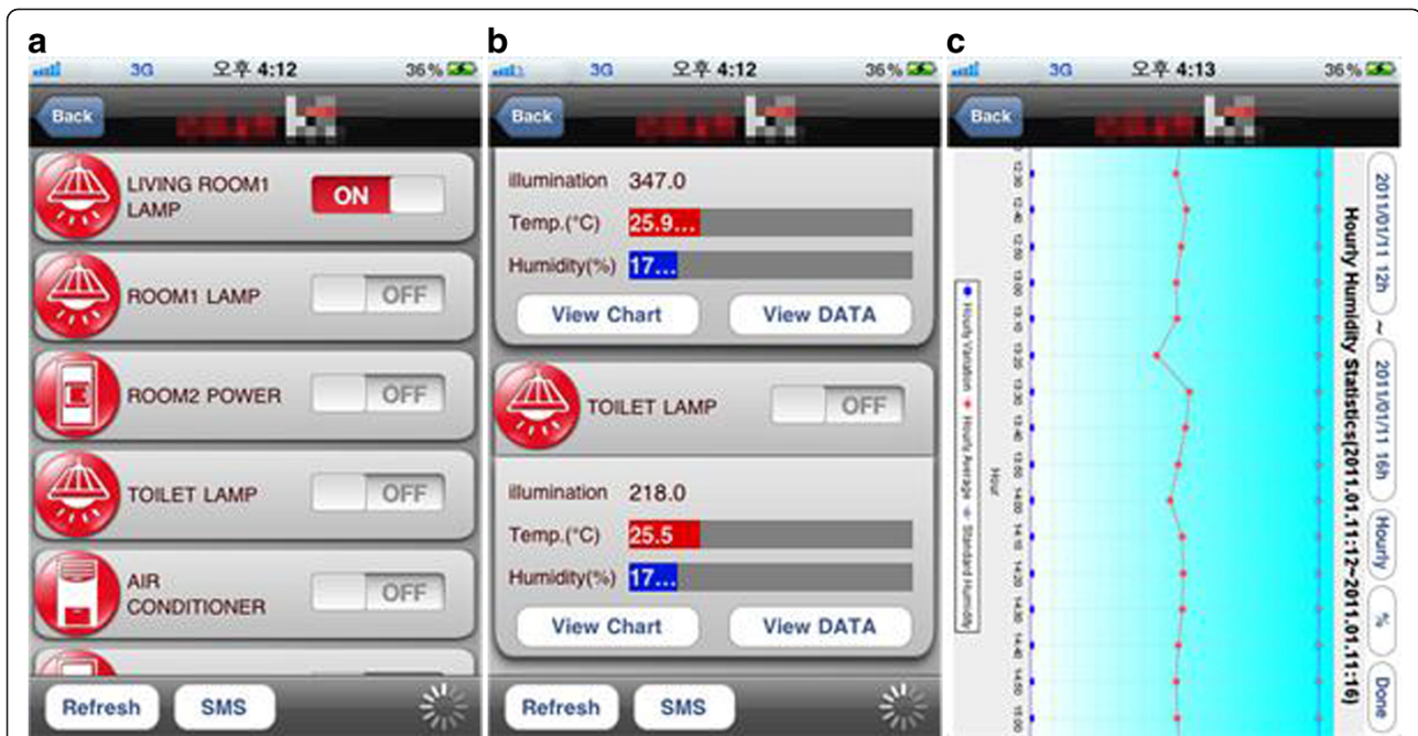
Figure 8 User interface to application: smart phone application interface. (a) Remote control. (b) Sensing information monitoring. (c) Statistical view of accumulated data.
