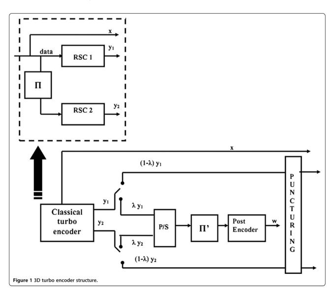
The choice of the post-encoder influences also the performance in both the waterfall and error floor regions. It has to meet different requirements already detailed in [2,3,6]. In [7], we justified the choice of the post-encoder by means of EXIT analysis. A four-state binary convolutional encoder is used in practice. The RSC code with feedback polynomial  $1 + D^2$  and parity generator polynomial 1 has been selected to be the post-encoder in different simulations of the 3D TC.
