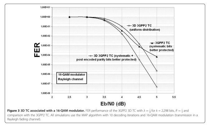
configuration 2, as in the example presented above for the 8-PSK. When the systematic bits are first protected as a priority and, if possible, the post-encoded bits, a significant gain is obtained. The technique is all the more interesting as the coding rates are higher for the same value of  $\lambda$ , even for transmissions over fading channels. In other words, the problem related to the loss in the convergence threshold of 3D TCs can be solved.
