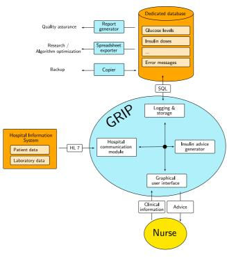
**High-level overview of GRIP**. Grip contains four major components: a component to interface with the hospital information system, a component to interface with the nurse, a component that calculates the advice that GRIP gives, and a component that logs errors and stores all data GRIP generates. HL7 : Health Level 7. SQL : Standard Query Language.
