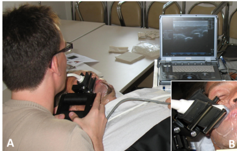
Figure 1 3D ultrasonographic examination of facial muscles. The linear array transducer was attached to a motorized 3D US acquisition system driven by a custom built linear mover connected to a laptop computer (A). Details of the attachment of the transducer to the 3D acquisition system are shown in (B).
