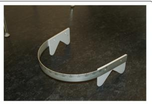
Figure 2 Device for the measurement of rotation ROM.
