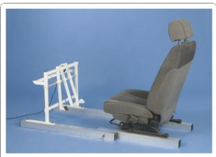
Figure 2 Custom-made apparatus to measure brake response time.
