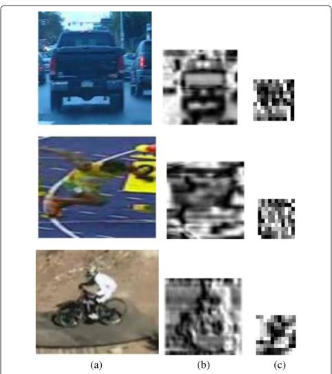
Fig. 3 Foreground response maps predict using different VGG feature maps. (a) Input image. (b) Using Conv4-1 feature only. (c) Using the concatenation of Conv4-2 and Conv4-3 feature with the proposed adversarial learning with attention
