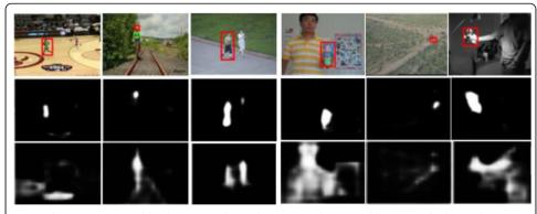
**Fig. 9** The maps generated by the proposed spatial attention scheme (middle row) and saliency detection algorithm [63, 64] Deep Saliency (bottom row)
