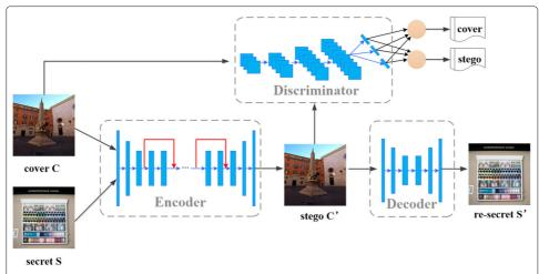
**Fig. 1** The architecture of HIGAN. The whole steganography model is composed of sub-networks: encoder, decoder, and discriminator. Encoder could hide a secret color image into a cover color image with the same size. The steganographic images generated by encoder are used as the input of the decoder, and then, the secret images are extracted by decoder. Discriminator takes the cover images and steganographic images as input to distinguish whether the input images contain secret images
