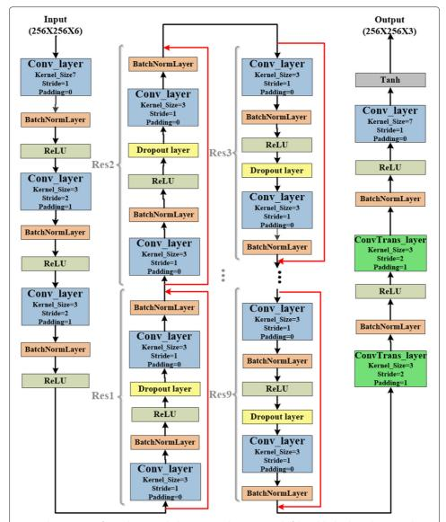
**Fig. 2** The structure of encoder network The entire work is composed of three blocks: three downsampling layers, nine residual layers, and three upsampling layers. In the downsampling phase, the channels of image gradually increase from 6 to 256. In the residual layers, the channels and size of feature maps are maintained at 256 and 64. In the upsampling layers, the channels of feature maps gradually reduce from 256 to 3
