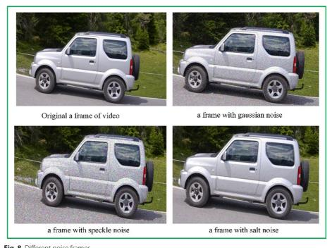
Fig. 8 Different noise frames
