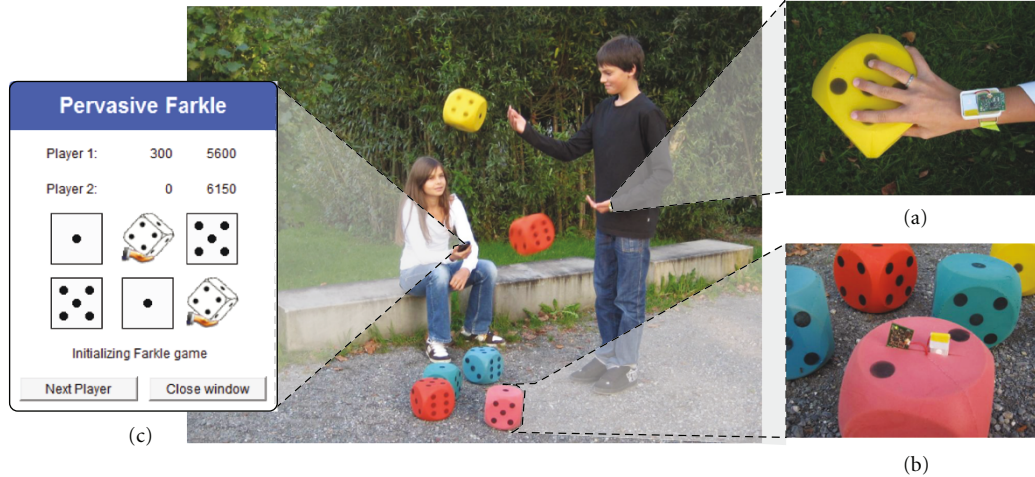
FIGURE 5: Two children wearing wristbands (a) playing the dice game with the smart dice (b). The game score is automatically updated on the mobile phone’s screen (c). Titan nodes with accelerometers are worn on the wrist (a) and integrated in the dice (b).
