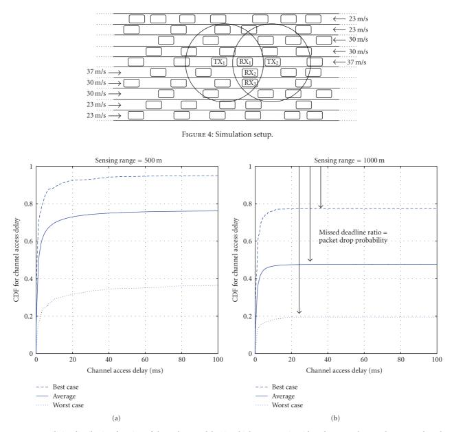
FIGURE 5: Cumulative distribution function of channel access delay, in a highway scenario with 10 lanes, 500 byte packets, 10 Hz heartbeat. (a) Sensing range of 500 meters and (b) sensing range of 1000 meters.
