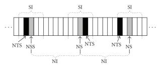
FIGURE 3: The frame structure for one node. The NSS and NSs are equally spaced with an interval of size NI. The SI parameter is also fixed.
