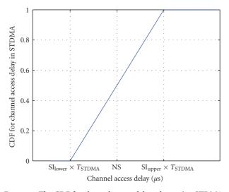
FIGURE 7: The CDF for channel access delay when using STDMA.
