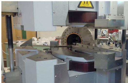
**Figure 4** Permanent Magnet in the high energy spectrometer with upper yoke lifted during assembly at Lalonde. Note the small size of the trim coil compared with the space available for a water-cooled full power coil
