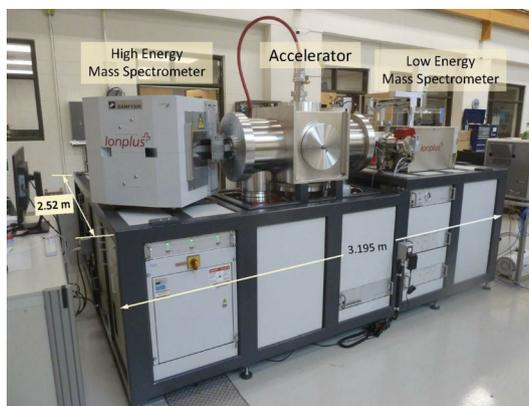
**Figure 3** Single Element  $^{14}\text{C}$  System installed at Lalonde AMS
