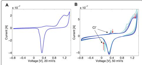
**Figure 2 Electrochemical cleaning protocol on gold coated cantilever in 50 mM KClO<sub>4</sub>.** Cyclic voltammogram in 50 mM KClO<sub>4</sub> (vs. Ag/AgCl (sat. KCl)). **A**, the standard gold spectra is shown at 20 mV/sec indicating a clean gold surface. **B**, a chloride contaminated surface is electrochemically cleaned. After six full potential sweeps, the chloride peaks vanish and a clear distinct gold reduction peak is observed.
