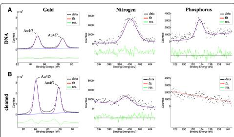
**Figure 4 XPS** measurements of the electrochemical removal of an oligonucleotide functionalization layer on the gold sample. X-Ray Photoelectron Spectroscopy (XPS) data are shown for the Au4f, N1s and P2p peaks for oligonucleotide functionalized **(A)** and electrochemical cleaned **(B)** gold samples. A clear increase in the gold peak as well as a clear removal of the phosphate peak of the cleaned sample can be seen.
