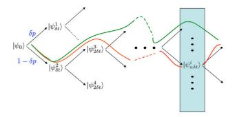
Fig. 5. Schematic representation of the time evolution of different quantum jump trajectories in the unraveling approach. At each time step, a quantum jump occurs with probability  $\delta p$ , and no event is observed with probability  $1 - \delta p$ . An ensemble of quantum trajectories provides an ensemble of pure states  $|\psi_{n\delta t}^i\rangle$  at time  $t = n\delta t$ , which is a valid decomposition of the density matrix at that time.
