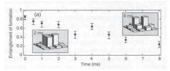
Fig. 1. Time evolution of the entanglement of a maximally entangled two-qubit state under environment coupling [20]. The insets show the statistical operator representing the quantum state at different times. While entanglement decays monotonously, the coherences of the density matrix are redistributed, but not clearly damped out. This highlights the nonlinear dependence of the state's entanglement on the statistical operator (Courtesy of C. Roos).
