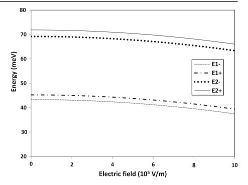
**Fig. 6** Plot of the energies  $E_{100}$ ,  $E_{111}$  against the electric field F. The energies have been calculated in the presence of the Rashba effect using Eq. (40). The parameters used in the calculations are given by Eq. (59)
