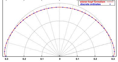
Fig. 4. Angular albedo pattern from weakly absorbing medium; single scattering albedo  $\omega = 0.99$ , incident  $\theta_0 = 45 \text{ deg}$ ; pattern angle  $\vartheta$  measured from exterior normal in x-y plane.
