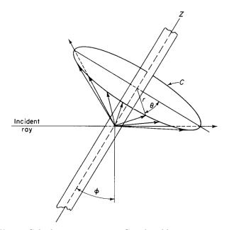
Fig. 1. Cylinder scattering cone C under oblique ray impact.
