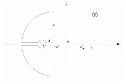
**Fig. 2.** Contour deformation for calculating  $\kappa_{-}(s)$ .
