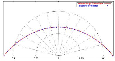
Fig. 3. Angular albedo pattern from strongly absorbing medium; single scattering albedo  $\omega = 0.60$ , incident  $\theta_0 = 45 \text{ deg}$ ; pattern angle  $\vartheta$  measured from exterior normal in x-y plane.
