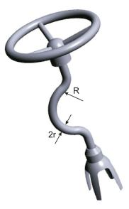
Fig. 3. Conceptional view of the C-shape memory prosthesis of the middle ear made of SMA.
