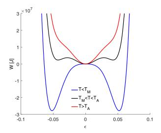
Fig. 4. Free energy of SMA spring at different temperatures according to Falk's model.
