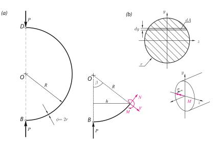
Fig. 5. Analytical model of the half-ring middle ear system prosthesis.
