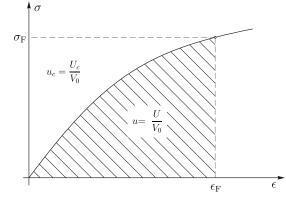
Fig. 6. Strain energy and complementary strain energy densities for an axial strain.
