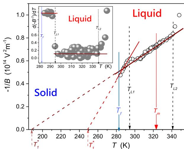
**Fig. 6** The temperature evolution of the negative reciprocal of the Kerr constant in liquid thymol.  $B$  (birefringence) denotes the EKE constant. Indicated temperatures are associated with melting, freezing, and changes in the temperature evolution. The parameterization is related to Eq. (3). The inset shows the derivative of experimental data from the central part of the plot, related to Eq. 4
