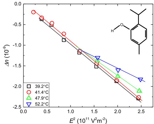
**Fig. 4** The plot shows the Kerr effect condition: anisotropy of the refractive index linear versus the square of electric field intensity in the tested sample at 312.3 K. On moving from the melting temperature, higher electric field were applied to obtain the response. The molecular structure of thymol is also shown
