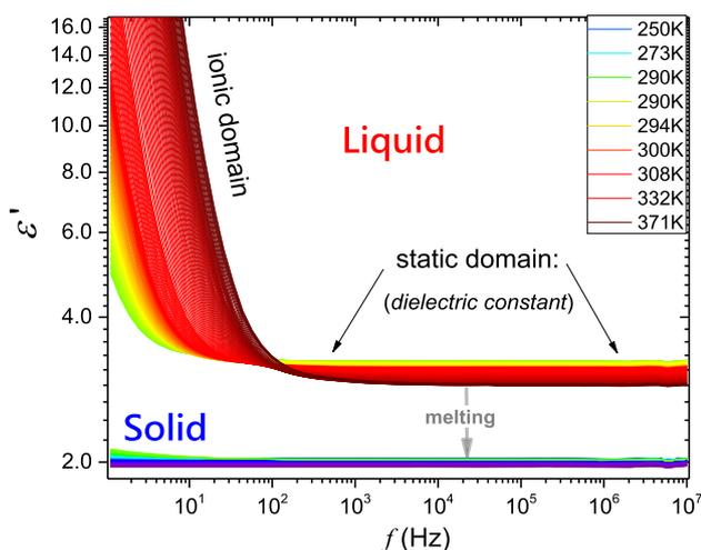
**Fig. 1** The frequency dependence of the of real part of dielectric permittivity in the tested temperature domain. Characteristic features of the spectrum are shown, including the manifestation of the melting phase transition
