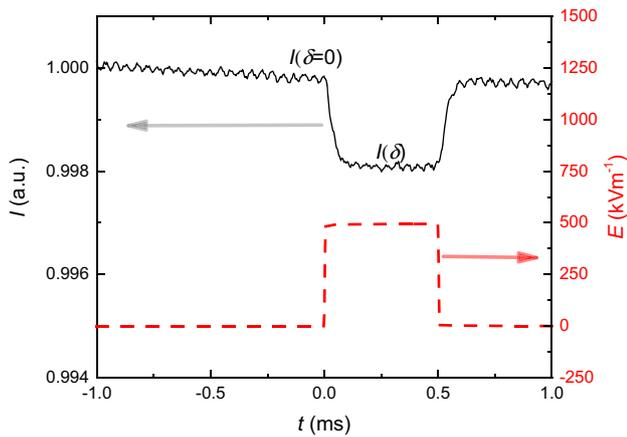
**Fig. 3** The shape of the detected photodiode current response (black, continuous line) of the sample to the pulse of the strong electric field (red, dashed line) measured at 327.3 K for impulses of 500 kV/m. Current values when no electric field was applied ( $I(\delta = 0)$ ) and when maximum electric field ( $I(\delta)$ ) was applied are marked
