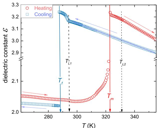
**Fig. 5** The temperature dependence of dielectric constant on heating and cooling, as indicated by arrows. The melting and freezing discontinuous phase transitions temperatures are indicated. Dashed vertical arrows indicate changes in the form of the temperature evolution. *Note:*  $T_f = 288.1$  K,  $T_m = 322.8$  K,  $T_{L1} = 294.0$  K, and  $T_{L2} = 330.9$  K
