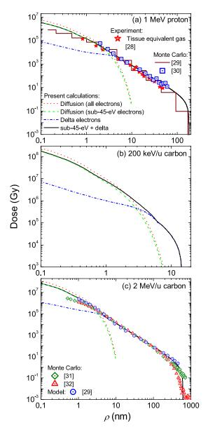
Fig. 2. Radial doses produced in liquid water by (a) a 1-MeV proton, (b) a 200-keV/u carbon ion and (c) a 2-MeV/u carbon ion. Lines correspond to the present calculations (see the text for details), symbols are the results from Monte Carlo simulations [29–32], and stars depict experimental data for tissue-equivalent gas [28].
