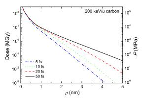
Fig. 1. Radial dose produced in liquid water by a 200-keV/u carbon ion as a function of time after ion traversal. Lines show present calculations using the diffusion equation for different times. The right axis represents the scale of pressure building up around the ion path.
