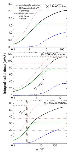
Fig. 3. Integral of the radial energy deposited in liquid water by (a) a 1-MeV proton, (b) a 200-keV/u carbon ion and (c) a 2-MeV/u carbon ion. Vertical dotted lines mark the radius  $\rho_{\Delta}$  corresponding to the restricted stopping power  $S_{\Delta}$  as defined in Section 4 (horizontal dotted lines). Horizontal dashed lines represent the unrestricted stopping power S of the ions (see the text for details).
