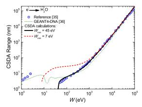
Fig. 4. Continuous slowing down approximation (CSDA) range of electrons in liquid water as a function of their energy for different electron thermalisation energies  $W_{\min}$  (solid and dashed lines). The dotted line represents GEANT4-DNA Monte Carlo results [36] while symbols are a compilation of reference data [35].
