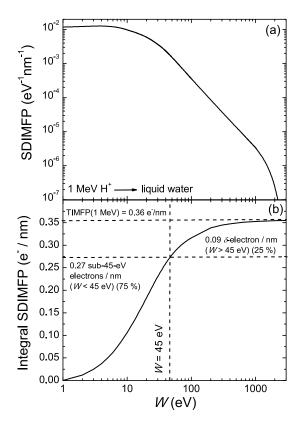
Fig. 5. (a) Ionisation singly differential inverse mean free path (SDIMFP) for 1-MeV protons in liquid water, and (b) integral of the SDIMFP as a function of the secondary electron energy W. Horizontal lines mark the total ionisation inverse mean free path (TIMFP) and the number of sub-45-eV electrons ejected per nanometer.
