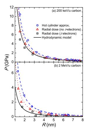
**Fig. 8.** Pressure on the wave front as a function of its radial position for (a) 200-keV/u and (b) 2-MeV/u carbon ions. Symbols are results from MD simulations, while lines correspond to the hydrodynamic model.
