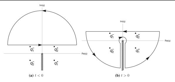
Fig. 1 Contour C that ensures causality, enclosing no poles for negative times. The branch cut is represented by the wavy line
