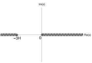
Fig. 2 Example of branch cuts starting at s = -3H and at the origin s = 0 and extending to the infinity
