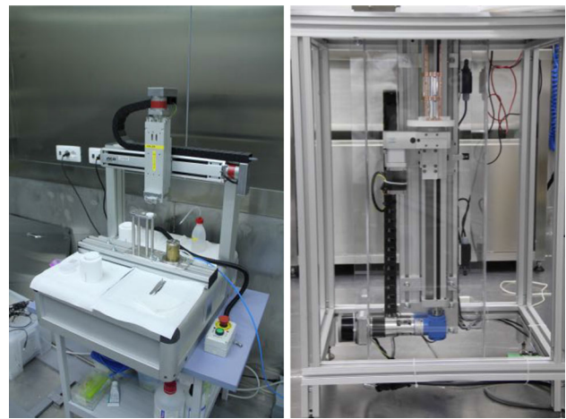
Fig. 11 Photos of the two working areas inside the cleanroom. On the left is shown the station where the Ge-NTD thermal sensors are glued to the absorbers, and on the right is shown the area where the towers are assembled
