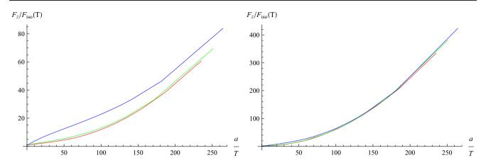
Fig. 13 Drag force in z direction as a function a/T at v = 0.5 (*left*) and v = 0.7 (*right*), where the *red*, *green*, *blue lines* represent Q = 0, Q = 1, Q = 2, respectively
