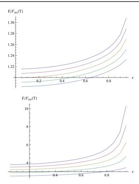
Fig. 9 The drag force F as a function of velocity for a quark moving through the plasma with Q = 2. The four graphs correspond to a/T = 1.38, a/T = 4.42, a/T = 12.2, a/T = 86, respectively, in
