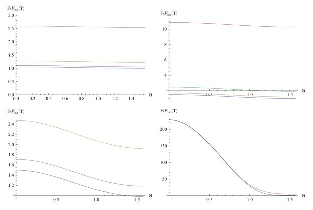
Fig. 7 Drag force F as a function  $\Theta$  at v = 0.9. The four graphs denote a/T = 1.38, a/T = 4.41, a/T = 12.2, a/T = 86, respectively, where the *color lines* denote Q = 5 (green), Q = 2 (brown), Q = 1 (red), Q = 0 (blue)
