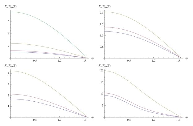
**Fig. 4** Drag force in z-direction  $F_z$  as a function  $\Theta$  at v = 0.5. The four graphs denote a/T = 1.38, a/T = 4.41, a/T = 12.2, a/T = 86, respectively, where the *color lines* denote Q = 5 (green), Q = 2 (brown), Q = 1 (red), Q = 0 (blue)
