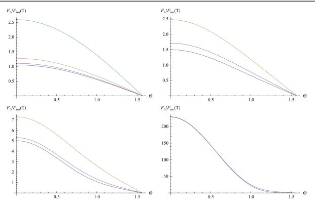
**Fig. 5** Drag force in z-direction  $F_z$  as a function  $\Theta$  at v = 0.9. The four graphs denote a/T = 1.38, a/T = 4.41, a/T = 12.2, a/T = 86, respectively, where the *color lines* denote Q = 5 (green), Q = 2 (brown), Q = 1 (red), Q = 0 (blue)
