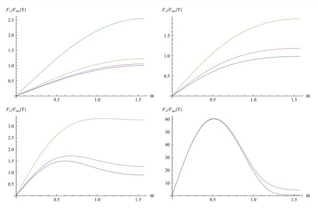
**Fig. 3** Drag force in x-direction  $F_x$  as a function  $\Theta$  at v = 0.9. The four graphs denote a/T = 1.38, a/T = 4.41, a/T = 12.2, a/T = 86, respectively, where the *color lines* denote Q = 5 (green), Q = 2 (brown), Q = 1 (red), Q = 0 (blue)
