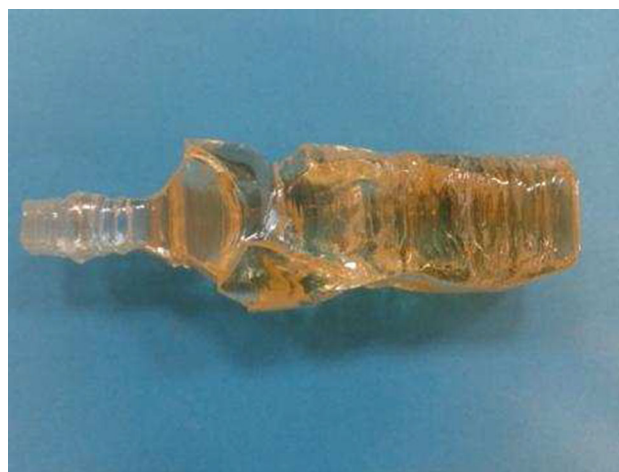
Fig. 1 Boule of \text{Zn}^{100}\text{MoO}_4 single crystal with mass of 170.7 g and length of 95 mm grown by the low-thermal-gradient Czochralski process
