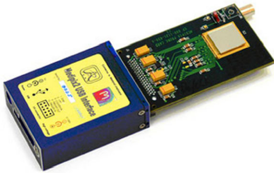
Fig. 1 The Timepix detector with a USB-Readout [9]
