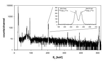
Fig. 1. Typical activation  $\gamma$ -spectrum taken after the irradiation of a natural Cd target with a 3.8 MeV proton beam. This spectrum was taken for 3 hours starting 8 minutes after the end of the irradiation. The inset shows the two resolved  $\gamma$ -peaks from the two reactions studied. The higher energy peaks visible in the spectrum are coming from beam-induced activities on heavier Cd isotopes.
