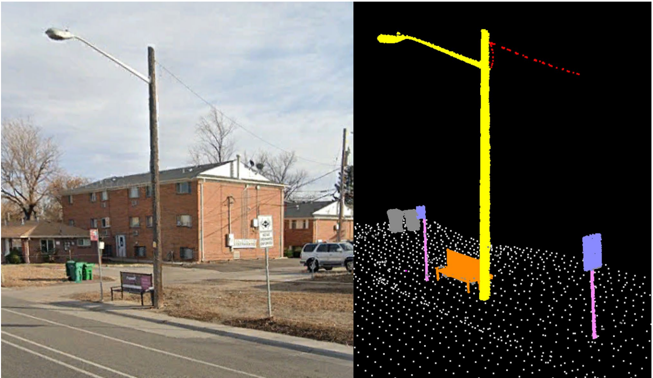
Fig. 4 Matching spaces in Google StreetView and Mobile LiDAR dataset
