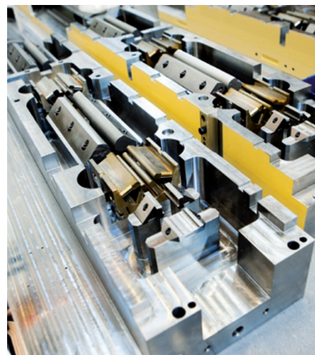
Magnets for the Swedish MAX IV synchrotron.
