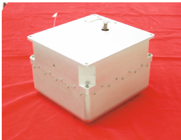
Figure 7. EGA instrument package.
