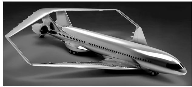
Fig. 1 Artistic representation of the PrandtlPlane object of study in the project PARSIFAL
