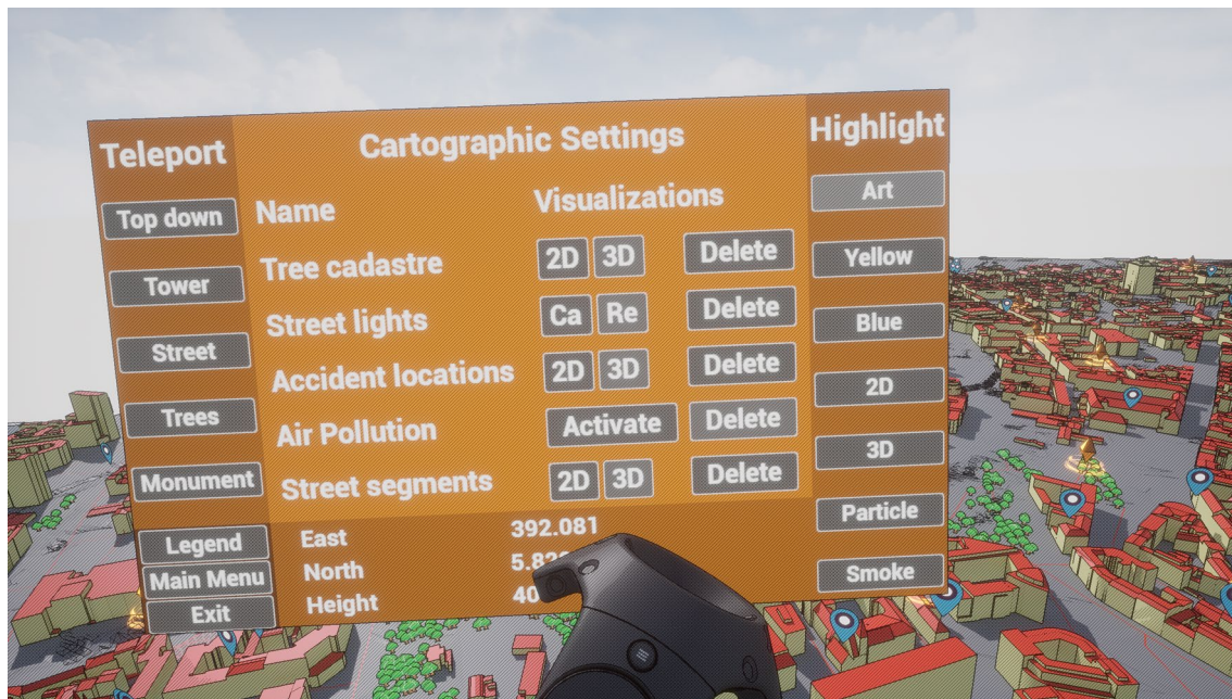
Fig. 9 An activated HUD with motion controls to change the visualization of the 3D scene
