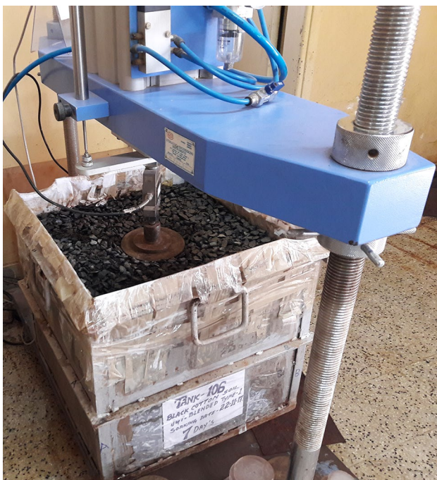
Fig. 2 Pavement model test in progress using cyclic loading machine
