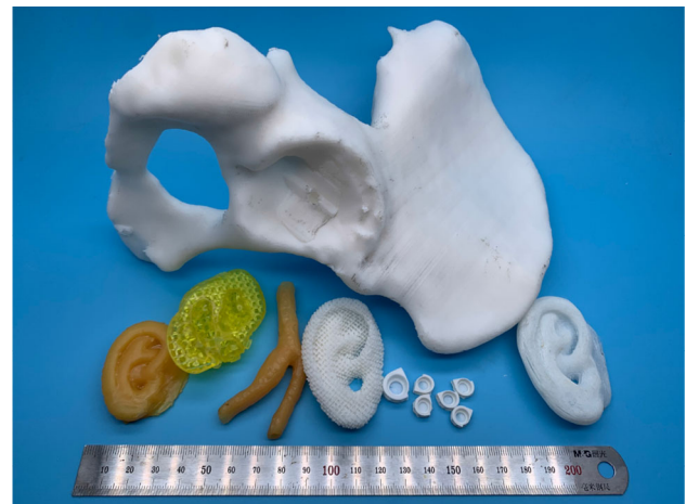
Fig. 3 Different 3D-printed polymers or polymer composites products. These polymer-based 3D-printed products have been studied for surgical models, surgical guide plates, artificial auricle stent, vascular stent, heart valve and so on. It shows good dimensional accuracy and mechanical properties
