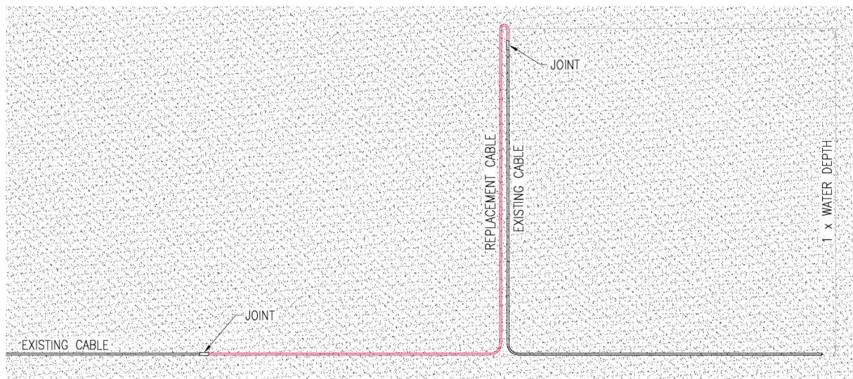
Fig. 9 HVDC cable route after repair—Omega loop
