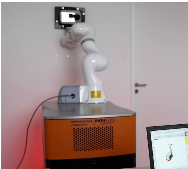
Fig. 13 An overview of the Kuka MKR iiwa mobile platform during a scan execution
