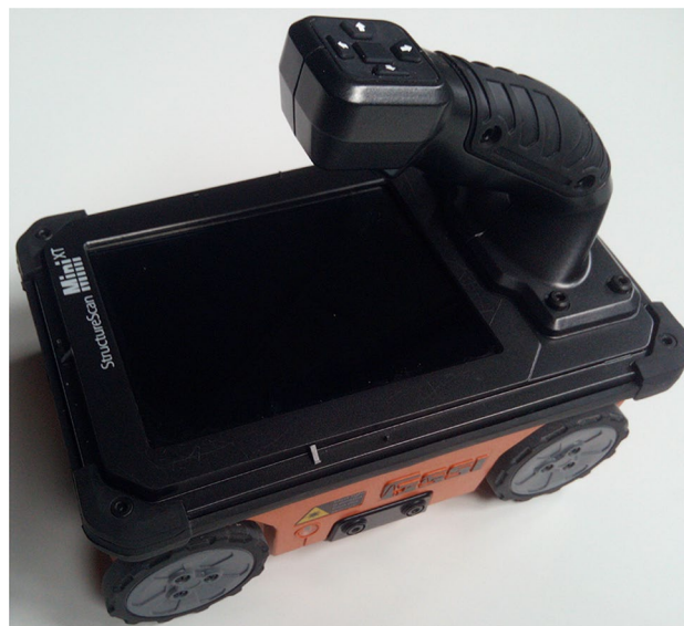
Fig. 2 Structure Scan Mini: a GPRdevice from GSSI developed for building structures
