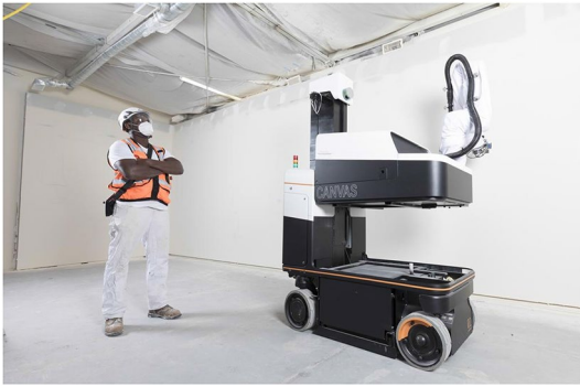
Fig. 9 Canvas drywall finishing robot
