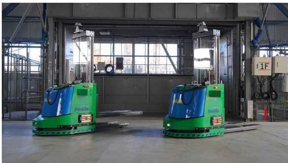
Fig. 4 Obayashi and Stocklin AGV material handling robots
