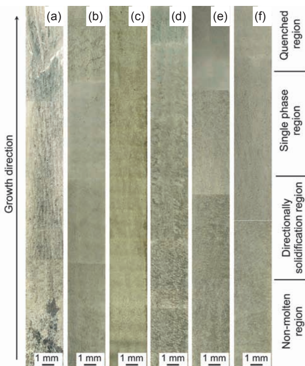
Fig. 3: Optical macrostructures of directionally solidified samples in longitudinal section at growth rate of 2 \mu\text{m}\cdot\text{s}^{-1} (a), 5 \mu\text{m}\cdot\text{s}^{-1} (b), 10 \mu\text{m}\cdot\text{s}^{-1} (c), 20 \mu\text{m}\cdot\text{s}^{-1} (d), 40 \mu\text{m}\cdot\text{s}^{-1} (e), and 50 \mu\text{m}\cdot\text{s}^{-1} (f), respectively, under a constant temperature gradient of G=18\text{ K}\cdot\text{mm}^{-1}
