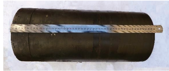
Fig. 1: Ti-44Al-8Nb-0.2W-0.2B-0.5Y alloy ingots fabricated by VAR
