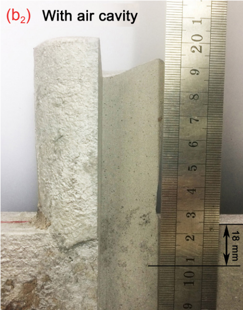
Fig. 7: Experimental results of insulation effect of air cavity on riser: (a) experimental temperature of Point B; (b) results of shrinkage; (c) cooling curves of Point 1
