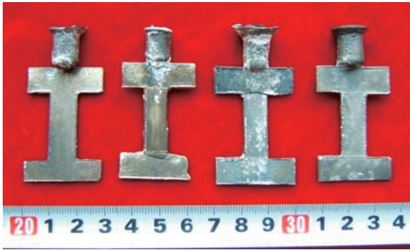
Fig. 6: Ti-47.5Al-2.5V-1Cr I-shaped specimen castings with different fibers addition in shell mold: (a) glass fibers; (b) carbon fibers; (c) without fiber addition; (d) nylon fibers [20]
