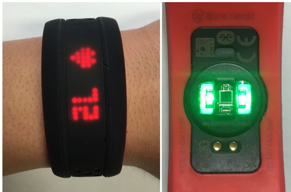
Fig. 5 A MIO Fuse and its PPG sensor
