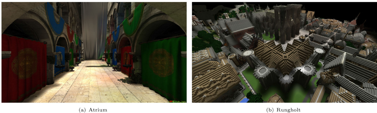
Fig. 1 Indirect lighting using VPLs with a small indoor Atrium scene and large outdoor Rungholt scene.
