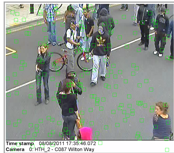
Fig. 3 Extracting patches at random is unreliable for selecting sufficient training patches to yield a good search results. Only 1 of 200 randomly placed patches will extract any of the Adidas® logo on the black hoodie.
