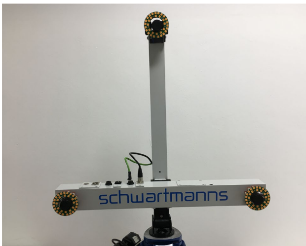
Fig. 1 Three-camera measurement system (horizontal/vertical base: approx. 650 mm)
