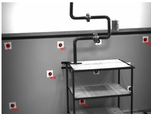
Fig. 17 Measurement constellation with pipeline and control points for analysing the reconstruction accuracy and the transformation quality
