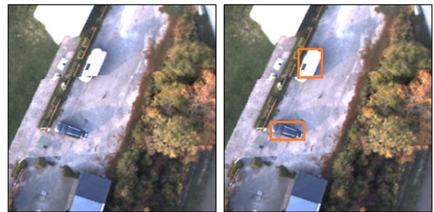
Fig. 11 On the left image, the input image tile is shown, whereby the image on the right side shows the representative object detection results on the tiling output for the Vehicle category (orange)
