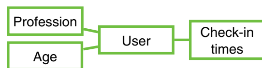
Fig. 1 Example schema of users and check-in times. Additionally, we know the age and profession of the users. There are three relationship types: there are relationships between (1) users and check-in times, (2) users and ages, and (3) users and professions
