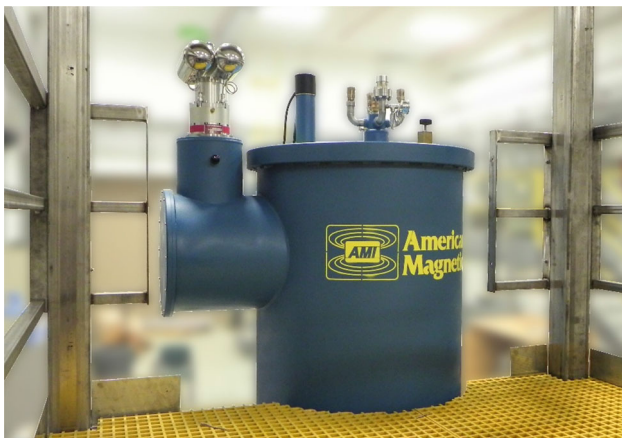
Figure 1. ORNL's 5-in. diameter, vertical warm-bore 9-T superconducting magnet system used for the Al thermomagnetic processing experiments.
