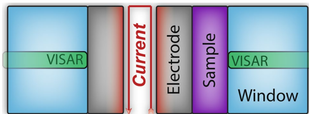
Fig. 1 One-dimensional configuration resulting from a typical Z strength experiment. Current flows between a pair of parallel electrodes and generates a magnetically driven ramp-release wave. The experimental observables are the velocity of the electrode/window interface on the left and sample/window interface on the right
