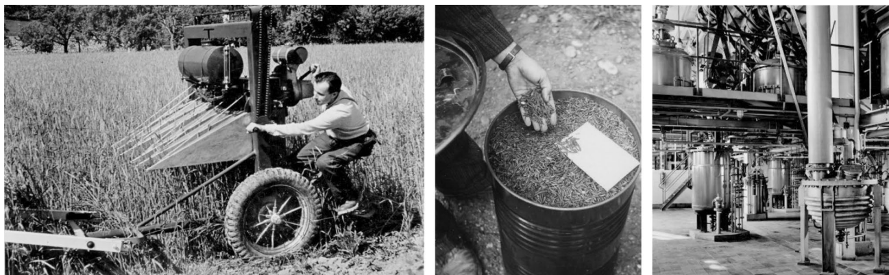
Fig. 27 Artificial inoculation of a rye field with the ergot fungus. Since the inoculation season usually coincided with the hay harvest, which tied up a lot of labor in agriculture, inoculation machines were developed. The ears were fed between the triangular dividers and inoculated with rollers studded with needles (left). In special cul-
