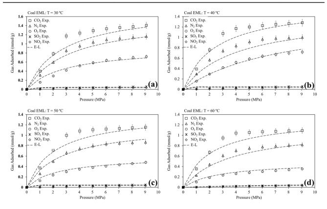
Fig. 8 Extended-Langmuir model fit for flue gas sorption on Coal EML at a 30 °C, b 40 °C, c 50 °C, and d 60 °C
