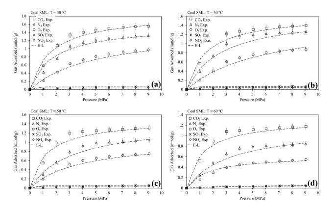
Fig. 9 Extended-Langmuir model fit for flue gas sorption on Coal SML at a 30 °C, b 40 °C, c 50 °C, and d 60 °C
