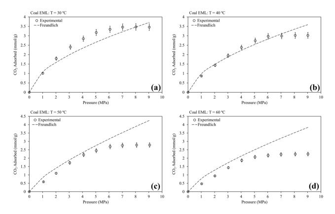
Fig. 3 Freundlich isotherm model fit for pure CO<sub>2</sub> sorption on Coal EML at a 30 °C, b 40 °C, c 50 °C, and d 60 °C
