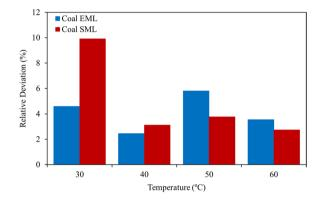
Fig. 11 Statistical comparison of experimental and theoretical maximum flue gas sorption capacity for **a** Coal EML and **b** Coal SML at 30 °C, 40 °C, 50 °C, and 60 °C
