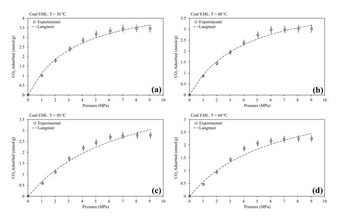
Fig. 1 Langmuir isotherm model fit for pure CO<sub>2</sub> sorption on Coal EML at a 30 °C, b 40 °C, c 50 °C, and d 60 °C
