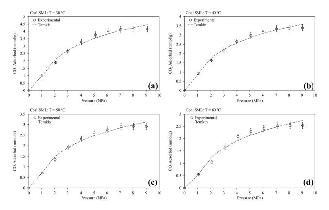
Fig. 6 Temkin isotherm model fit for pure CO<sub>2</sub> sorption on Coal SML at **a** 30 °C, **b** 40 °C, **c** 50 °C, and **d** 60 °C
