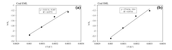
Fig. 12 van't Hoff plots for a Coal EML and b Coal SML
