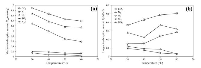
Fig. 10 Change curves of extended Langmuir parameters with temperature: a Maximum adsorption amount; b Langmuir adsorption constant for Coal EML
