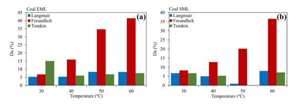
Fig. 7 Statistical comparison of experimental and theoretical maximum CO<sub>2</sub> sorption capacity for **a** Coal EML and **b** Coal SML at 30 °C, 40 °C, 50 °C, and 60 °C
