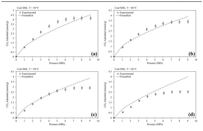
Fig. 4 Freundlich isotherm model fit for pure CO<sub>2</sub> sorption on Coal SML at a 30 °C, b 40 °C, c 50 °C, and d 60 °C
