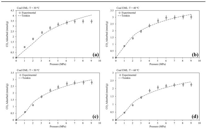
Fig. 5 Temkin isotherm model fit for pure CO<sub>2</sub> sorption on Coal EML at a 30 °C, b 40 °C, c 50 °C, and d 60 °C
