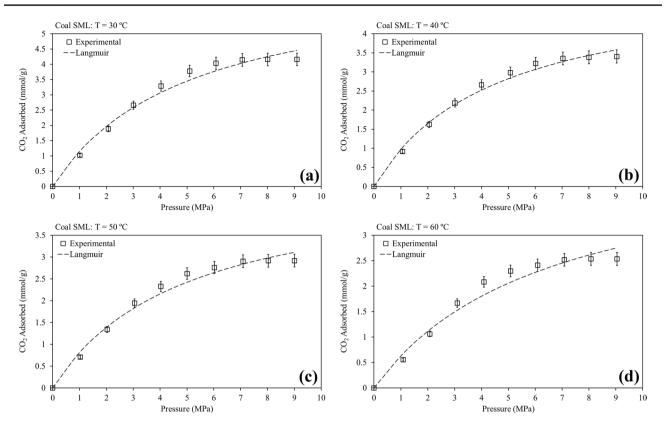
Fig. 2 Langmuir isotherm model fit for pure CO<sub>2</sub> sorption on Coal SML at a 30 °C, b 40 °C, c 50 °C, and d 60 °C
